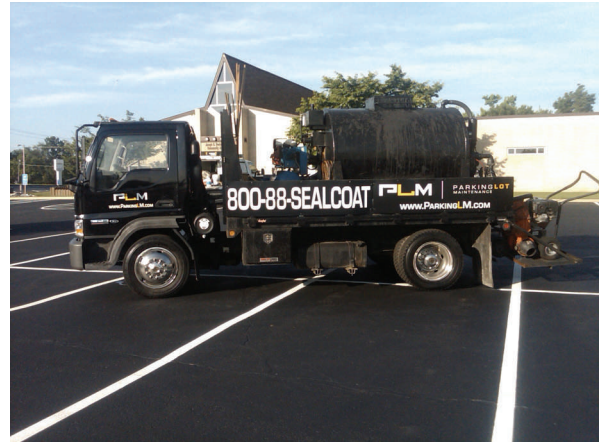
This 700 gallon truck mounted tank owned by Parking Lot Maintenance has a "Full Sweep" agitating system.
